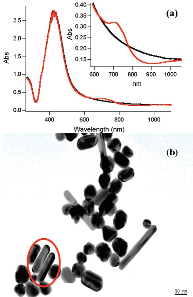
**Figure 1.** (a) Absorbance of colloidal silver nanoparticles dispersed in water. Solid black line, initial spectrum before exposure to 800 nm radiation; red line, after exposure to radiation for 60 min. The inset magnifies the observed change in the spectrum. (b) TEM image of the silver nanoparticles used in the experiment shows a broad dispersion in size and shape. The experiment selects rods with dimensions that are consistent with the two nanorods seen in the lower left corner of the image.
