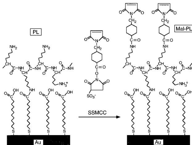
Figure 5. Reaction scheme showing the attachment of maleimide groups to the PL-coated surface. The covalently attached PL monolayer is reacted with an NHSS–maleimide molecule, SSMCC, to form a maleimide-modified poly(L-lysine) (Mal-PL) layer.
