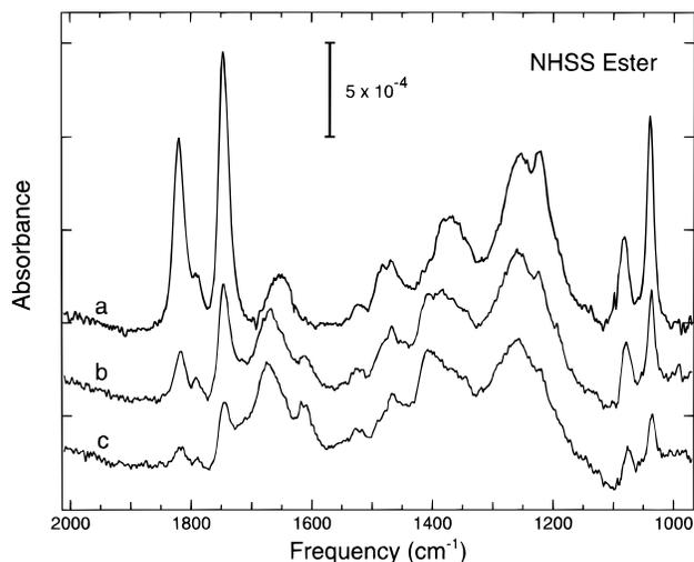
Figure 3. PM-FT-IRRAS spectra of the intermediate NHSS ester layers for the same sample used in Figure 2. (a) NHSS ester monolayer obtained in the first reaction cycle of the MUA SAM with EDC/NHSS. (b) NHSS ester layer from the second cycle. (c) NHSS ester layer from the third cycle. The 1820 cm<sup>-1</sup> band signifies the formation of MUA-NHSS esters as opposed to merely adsorption of NHSS onto the surface (see Table 1 for band assignments).
