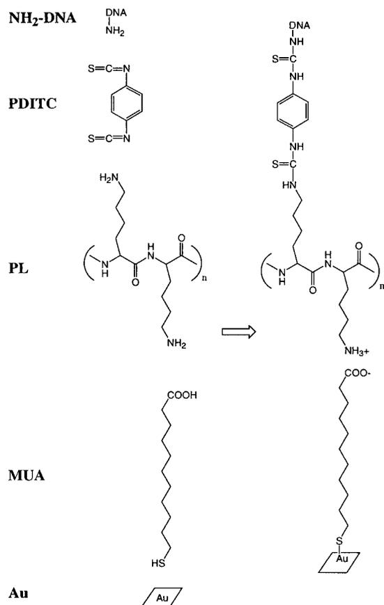
Figure 1. Schematic of method used for coupling 5'-amine-terminated oligonucleotide probes to a gold surface.
