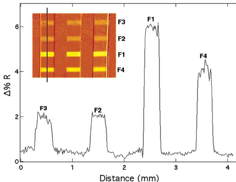
Figure 6. SPR difference image showing the binding of 100 nM solution of anti-FLAG M2 to a peptide array. The line profile shows the differential binding of antibody to the original sequence (F1) and peptide variants produced by replacing one of the original residues with alanine (F2, F3, F4). The peptide sequences are listed in Table 1.
