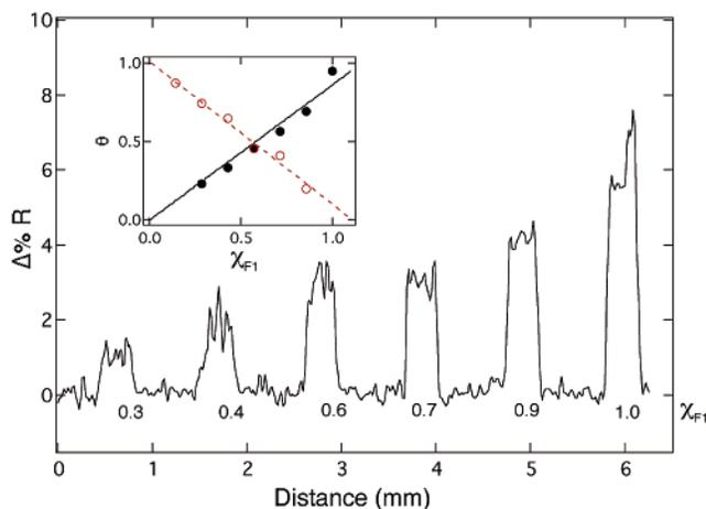
Figure 5. Line profile showing the adsorption anti-FLAG M2 (50 nM) onto a peptide array composed of F1 peptide diluted into the noninteracting HA peptide in mole fractions ranging from 0.29 to 1.00 F1. The graph inset shows the antibody surface coverage obtained when the array is exposed sequentially to anti-FLAG (●) and 10 nM anti-HA (○).
