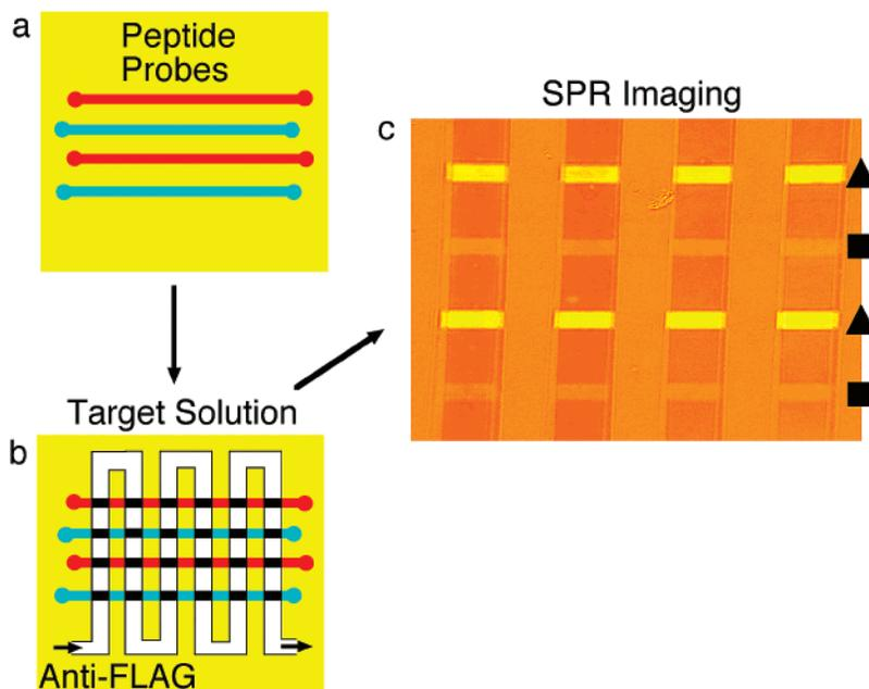
Figure 2. Schematic drawing showing fabrication of a peptide array on a gold surface. (a) A set of parallel PDMS microchannels was used to immobilize peptides onto a gold film, (b) A second PDMS microchannel was used as a small-volume sample cell ( $5 \mu\text{L}$ ) to deliver target molecules (e.g., antibody) to the peptide line array. (c) SPR difference image showing the adsorption of anti-FLAG M2 onto a two-component peptide array.
