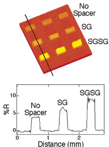
Figure 3. SPR difference image showing the binding of a 100 nM solution of anti-FLAG M2 to a peptide array composed of peptides containing the F1 sequence (refer to Table 1) modified with either an SGSG spacer, an SG spacer, or no spacer. The most antibody adsorption was observed at the peptide with the SGSG spacer.
