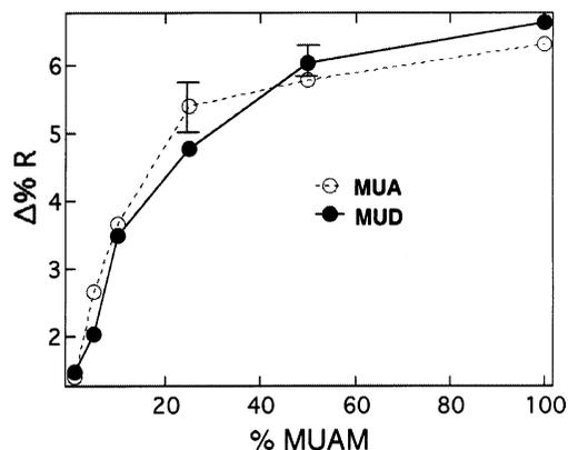
Figure 4. Comparison of the change in percent reflectivity upon anti-FLAG adsorption (100 nM) onto F1 peptide arrays fabricated on mixed monolayers containing various percentages of MUAM in MUA (○) and MUAM in MUD (●). Representative error bars have been included for these measurements. The dotted and solid lines are included as an aid to the eye.
