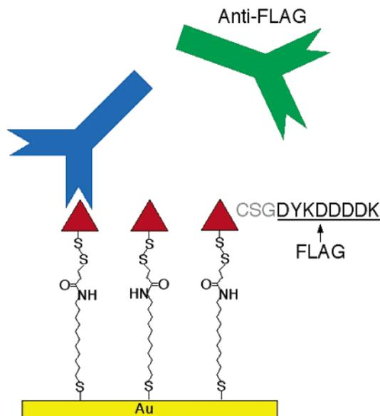
Figure 1. Schematic diagram illustrating the chemical attachment of peptides on gold surfaces. FLAG peptides were modified with a terminal cysteine for direct attachment onto a self-assembled monolayer on gold via a sulfhydryl–disulfide exchange reaction. The FLAG sequences contained an SG spacer between the cysteine and the FLAG sequence to maximize antibody accessibility to the immobilized peptide.
