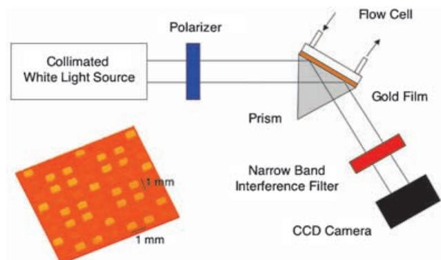
**Figure 1. Schematic diagram of a SPR imaging set-up**
