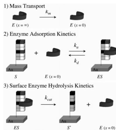
**Figure 1.** Reaction scheme showing the surface enzymatic processing of a biopolymer microarray including mass transport, enzyme adsorption onto a surface-bound substrate, and followed by a surface enzyme hydrolysis reaction.
