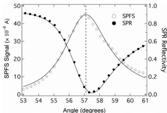
**Figure 5.** SPFS and SPR signals as a function of incident laser angle obtained for hybridization/adsorption of 500 nM fluorescently labeled RNA (AFR1) to surface-immobilized DNA (D1) probes. The SPR (●) and SPFS (○) curves were fitted using four-phase Fresnel calculations. The solid lines represent the fit. The dashed line corresponds to the angle position where the maximum fluorescence signal was achieved.
